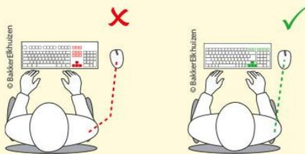
The distance between the keys ranges from 18 to 20 mm (ISO 9241). The alphabetical section must be clearly separated from the function keys (ISO 9241). Dark letters on a clear background are easier to read (ISO 9241) and contribute to an increased productivity (Snyder, 1990). The middle row of keys cannot be elevated more than 30 mm above the surface of the desk (DIN 2137). The keyboard must be tiltable and separate from the screen (Council Directive 90/270/EEC).
